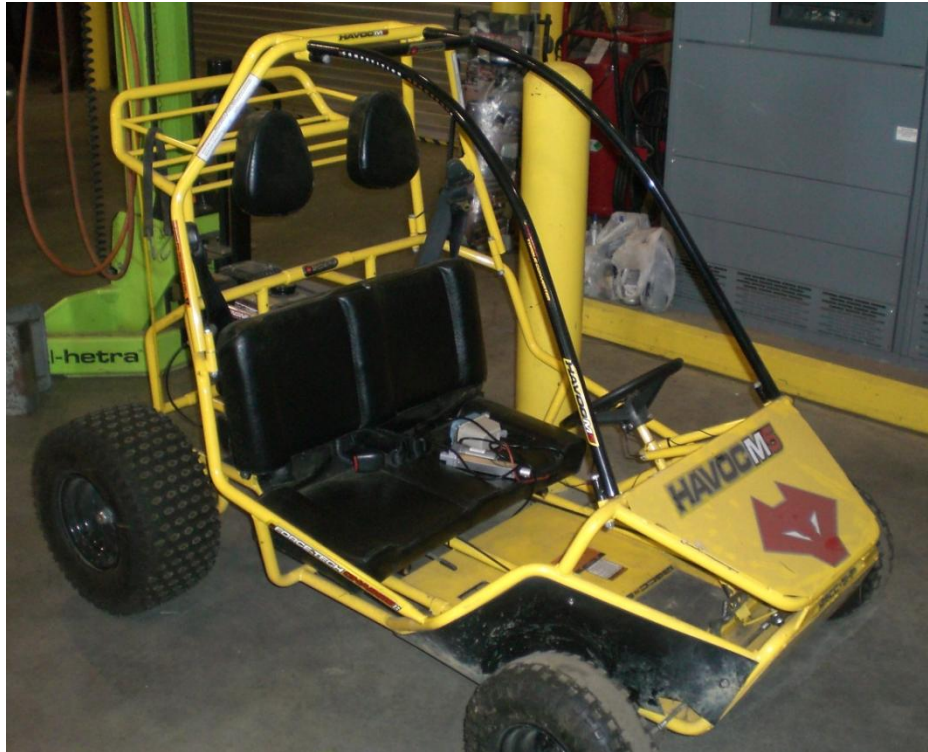
Figure 3.1: The Off-road Go-Kart Used as the Ground Vehicle Platform for Teleoperation
