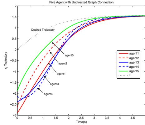
Fig. 6. Trajectory Tracking of 5 Agents with Undirected Graph
